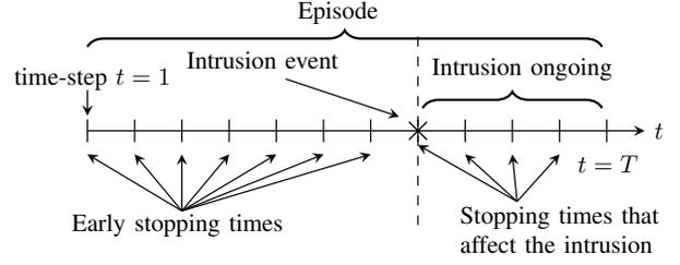
Fig. 3: Optimal multiple stopping formulation of intrusion prevention; the horizontal axis represents time;  $T$  is the time horizon; the episode length is  $T - 1$ ; the dashed line shows the intrusion start time; the optimal policy is to prevent the attacker at the time of intrusion.
